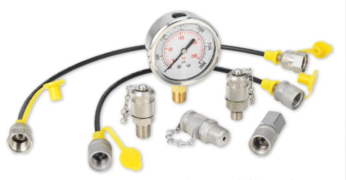
Anchor Fluid Power test point fittings allow for the safe and easy connection of gauges to monitor hydraulic system pressure. Gauges and hoses can be attached without tools and while the system is under pressure. Test point fittings can also be used for bleeding air from the system and taking fluid samples for analysis. An o-ring seals the protective metal cap to prevent contamination and loosening due to vibration.
